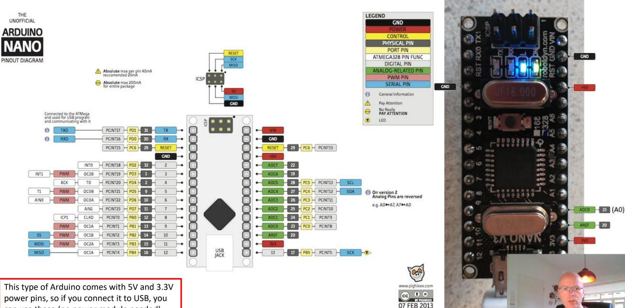
power pins, so if you connect it to USB, you can use these (no power module needed), you may also use this Arduino as a power module if you do not have one at hand ;-)
